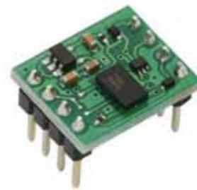
MMA7455 3-Axis Accelerometer
