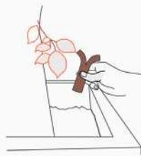
2. After charging is completed, leaf-sensor is placed into plant pot.
