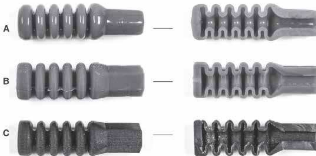
Fig. 4. Linear actuator design parameters (top) and fabricated Samples for A. RLP B. Silicone Casting and C. MMPP.
