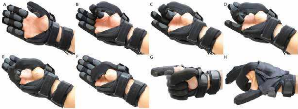
Figure 9. Range of motion of the soft robotic glove. A. Pretention of the fabric sleeves surrounding the fiber-reinforced actuators offers full hand extension. B-F. Executing the Kapandji test [21] with the soft robotic glove for thumb range of motion. G. Finger flexion with index finger straight. H. Index finger flexion.
