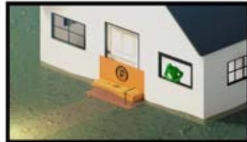
**Step 12:** Open both yellow valves and attach 3/8 inch garden hose attachment to garden hose. Fill water into either valve and close both valves once filling is complete. It's important to not overfill the tube. Do not fill the tube past the bottom of the top white pvc pipe.
